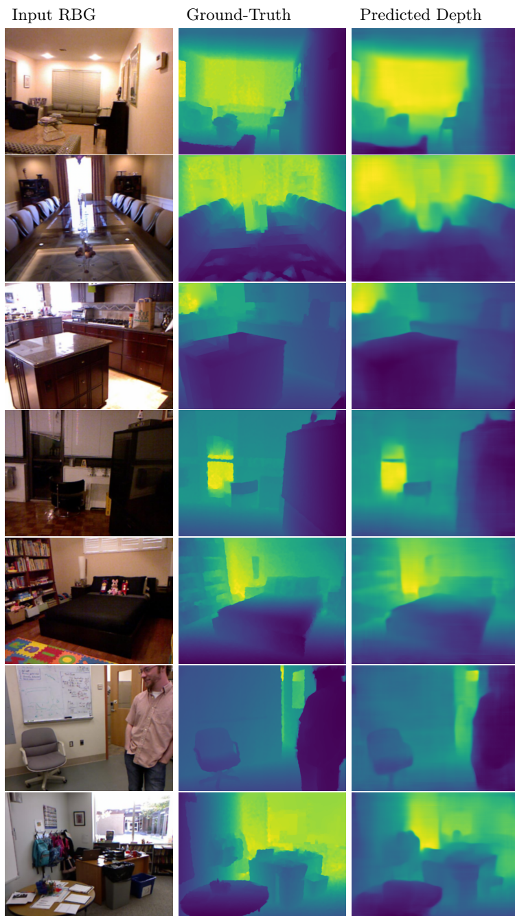
Figure 4. Output of our model on NYU RGB-D dataset. The first row shows the input RGB image, the second row shows the ground truth depth image, and the last row shows the estimated depth image of our method.
